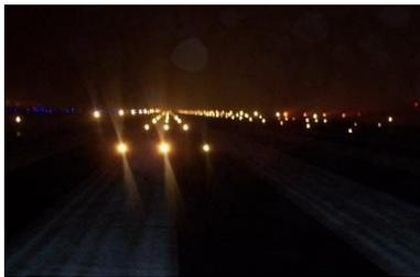
The Jetport has equipped Runway 11-29 with in-pavement lighting that provides additional visual references for departing and landing aircraft. For driver training purposes, know that these lights are actually flush with the runway's surface and are white or red in color.
