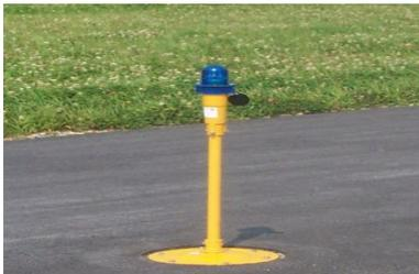
Taxiway edge lights are always blue in color. These lights are used at night and during bad weather conditions to illuminate the taxiway’s route and to delineate where the edges are located.
