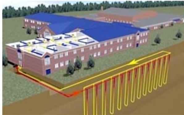
*Graphic representation of a geothermal system*
