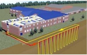
Graphic representation of a geothermal system
